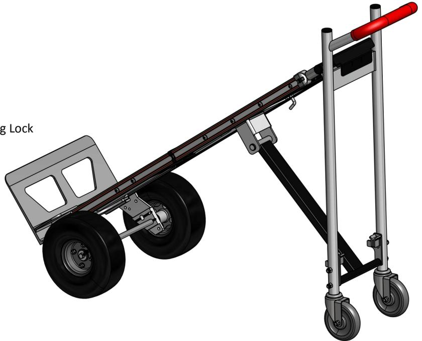
1. Unlock the 4th wheel from the frame, then pivot the assembly so the top of the frame handle contacts the cross member just below the red handle, causing the spring lock to engage into the hole.
